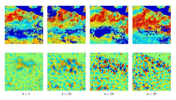
FIGURE 3. Real satellite sequence of SST (sea surface temperature) images. Dark blue regions indicate missing data due to the cloud cover or land regions. First row: SST images at different days k = 1, 10, 24, 39 and estimated velocity fields with the WETKF assimilation of image data; Second row: Mean estimated vorticity with WETKF and associated velocity fields.
